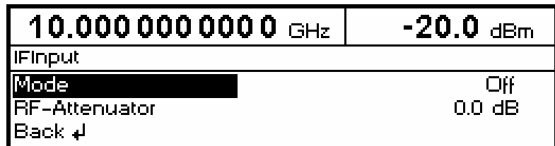
Fig. 4-19 IFInput menu (preset setting), option R&S SMR-B23/R&S SMR-B24 fitted
