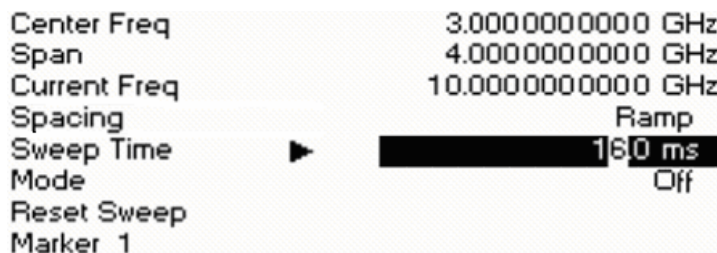
Fig. 4-24 Section of Sweep - Freq menu, example of Spacing Ramp (ramp sweep)
